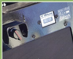
Stop switch for gasoline engine (MVH-308/408)
